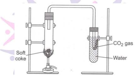
Then add blue lit mus solution (to test the formation of acid) to the test tube in which carbon dioxide gas is dissolved. The colour of the solution turns red. The following chemical reactions are going on during this experiment
