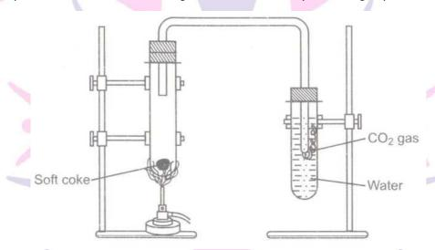
Then add blue lit mus solution (to test the formation of acid) to the test-tube in which carbon dioxide gas is dissolved. The colour of the solution turns red. The following chemical reactions are going on during this experiment.
